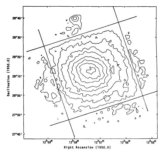
FIG. 2. - A contour plot of the X-ray surface brightness distribution for the Coma cluster observed with the IPC on board the Einstein Observatory. The superimposed lines represent the instrument's window support structure which distorts the image within 2' of the positions shown. The point source to the north of Coma is X Comae, a Seyfert galaxy.
