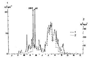
Fig.1. Variations of the daily suspended sediment concentrations (1) and the 10 days' mean sediment discharge (2) during the year. Vakhsh river, Tutkaul, 1956
