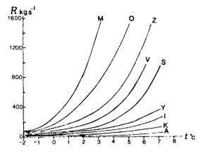
Fig.2. The monthly mean sediment discharge R for some glacier rivers versus the monthly mean temperature t at lednik Fedchenko meteorological station
