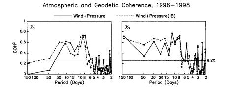
Figure 3. Coherence between geodetic and atmospheric terms (including or not including the IB effect) between 2 and 150 days. The horizontal line gives the measure of 95% significance.
