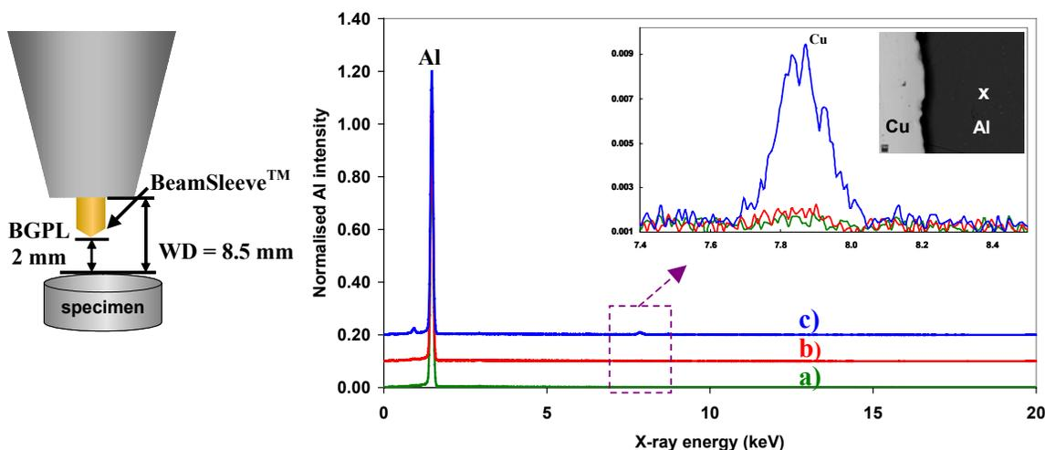
Fig 2 Left: BeamSleeve™ attached to the pole piece of the SEM, reducing the BGPL to 2 mm at the analytical working distance of 8.5 mm.
