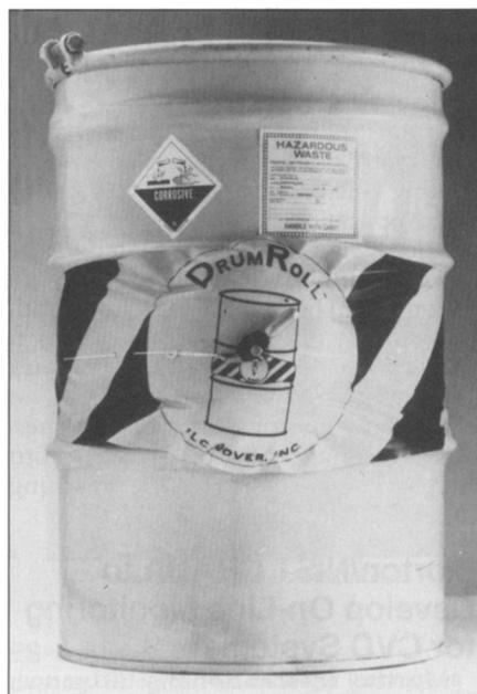
▲ **Inflatable Spill-Control Device:** The DrumRoll<sup>®</sup> from ILC Dover can stop 55-gallon-drum leaks that are up to 7" x 2" in size. To stop a leak, users wrap the device around the drum and pull the inflation cord. A CO<sub>2</sub> cartridge then inflates a chemically resistant Teflon-coated bladder which stops the leak. No tipping or pegging is required, and one person may operate the device alone. A reusable training kit includes a DrumRoll<sup>®</sup> that can be
