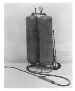
Figure 8. Double-tank pressure knapsack. This double-tank unit is constructed of stainless steel. It incorporates a tank valve, pop-off relief value and pressure gauge at the top. A quick-coupler injector and pressure regulator are installed at the bottom. The spray is dispersed through the regulator to the hose and gun. Nozzle pressure is 30 psi. Initial air pressure is 30 psi. When liquid is pumped in until the pressure reaches 100 psi, the liquid capacity is five gallons.
