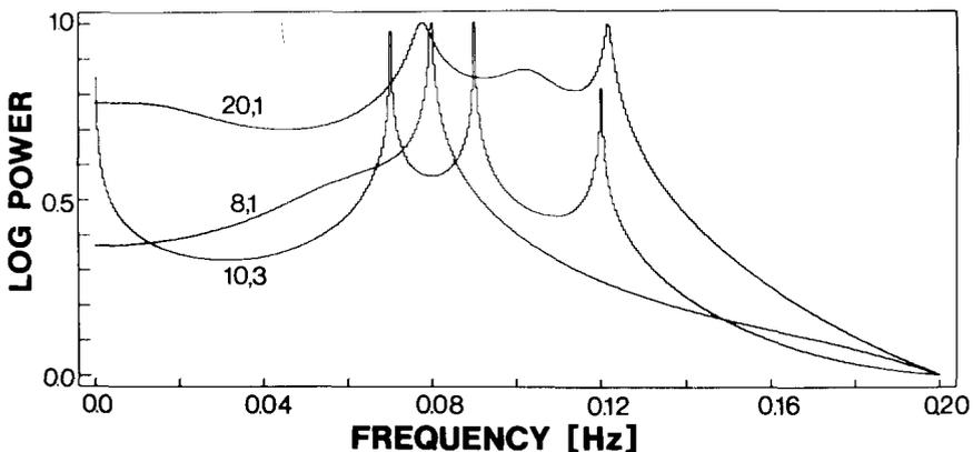
Fig. 1. LS AR spectra of a test signal with three sinusoidal components of different frequencies. The various filter order and averaging numbers are indicated near each curve (for details, see text).
