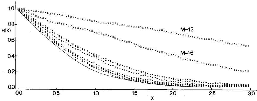
Fig. 3. Empirical probability distribution functions of the frequency shift when using the Fourier method (continuous line) and the LS AR spectral estimator (other symbols).  $H(x)$  means the probability that the value of  $\sqrt{N} N \Delta t |\Delta f| A / \sigma$  exceeds the value of  $x$  (for details see text).
