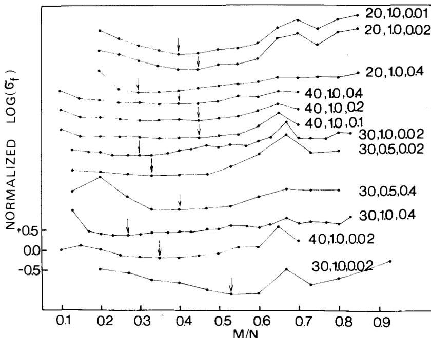
Fig. 2. Dependence of the standard deviation of peak location on the relative filter length ( $M/N$ ) for different signals (for details, see text).
