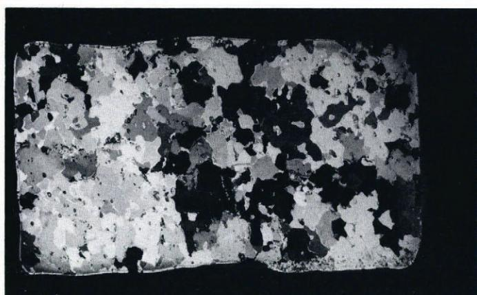
Fig. 10. Thin-section photograph of crystalline texture of ice specimen TC A4 between crossed polaroids after deformation in torsion-compression.  $\tau = 2.8$  bar and  $\sigma = 2.7$  bar; dimensions of the thin section: 8 cm  $\times$  4.6 cm. The torsion axis was parallel to the direction containing the largest dimension of the thin-section. The radial direction was perpendicular to the thin section.
