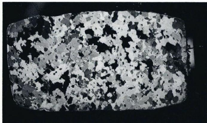
Fig. 9. Thin-section photograph of crystalline texture of ice specimen TC A2 between crossed polaroids after deformation in torsion-compression.  $\tau = 1.85$  bar and  $\sigma = 5.7$  bar; dimensions of the thin-section: 8 cm  $\times$  4.5 cm. The torsion axis was parallel to the direction containing the largest dimension of the thin section. The radial direction was perpendicular to the thin section.
