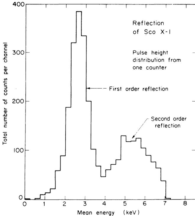
Fig. 2. Pulse-height distribution from one counter during observation of Sco X-1. The two peaks are caused by first- and second-order reflection of the continuum from the crystal. The upper and lower cut-offs in the transmitted data are at 7 and 1.5 keV.
