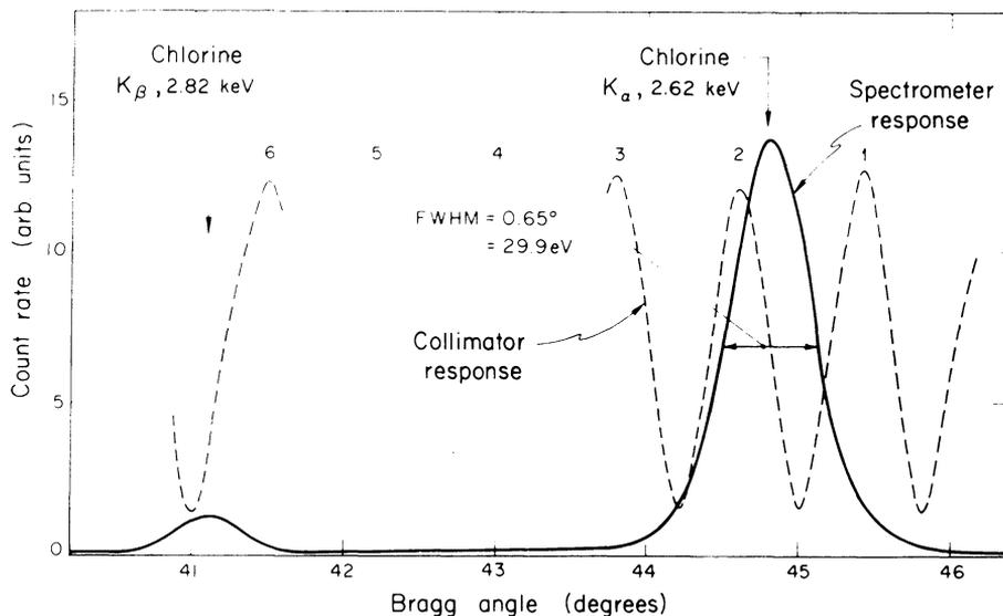
Fig. 3. Laboratory measurement of the reflection from one panel, showing peaks due to the  $K_{\alpha}$  and  $K_{\beta}$  lines of chlorine. The broken line shows the response of the modulation collimator detector permanently fixed to the crystal panel.
