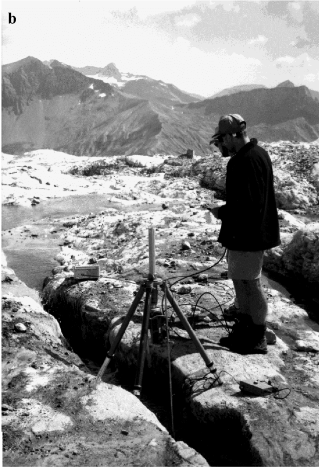
Fig. 1. (a) Map showing the margin of Glacier de Tsanfleuron, and the area of the recently exposed limestone glacier forefield. (b) Photograph of the Nye channel measured by an EDM showing the propeller current meter suspended by a tripod (taken from the ice margin looking across the limestone platform).
