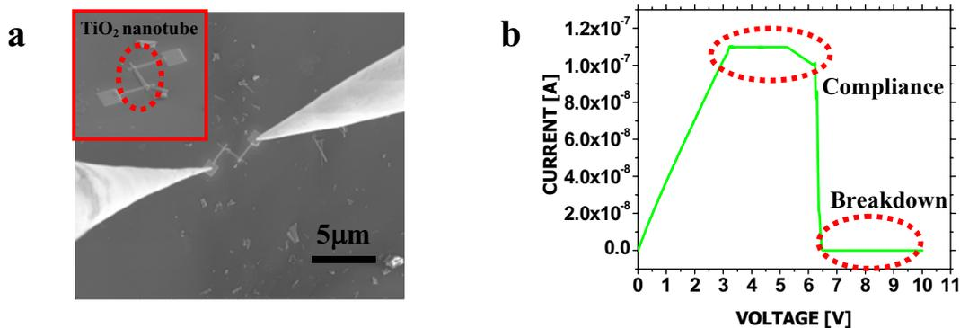
FIG. 1. (a) SEM image of W probes and TiO<sub>2</sub> nanotube electrical test structures fabricated by FIBID. (b) TiO<sub>2</sub> nanotubes with 200 nm diameter and 15 nm thick walls show semiconducting resistivity of an order of 1 ·Ωcm.
