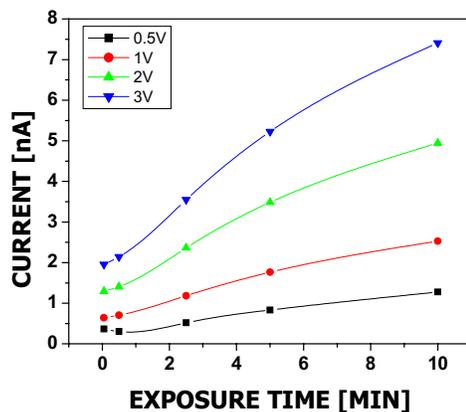
FIG. 3. I-V behavior with respect to E-beam exposure time.
