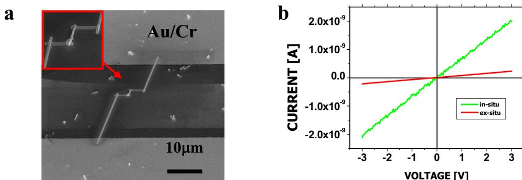
FIG. 2. (a) SEM image of TiO<sub>2</sub> nanotube test structure with the Au/Cr electrodes. (b) I-V measurement results: *in-situ* vs. atmosphere.
