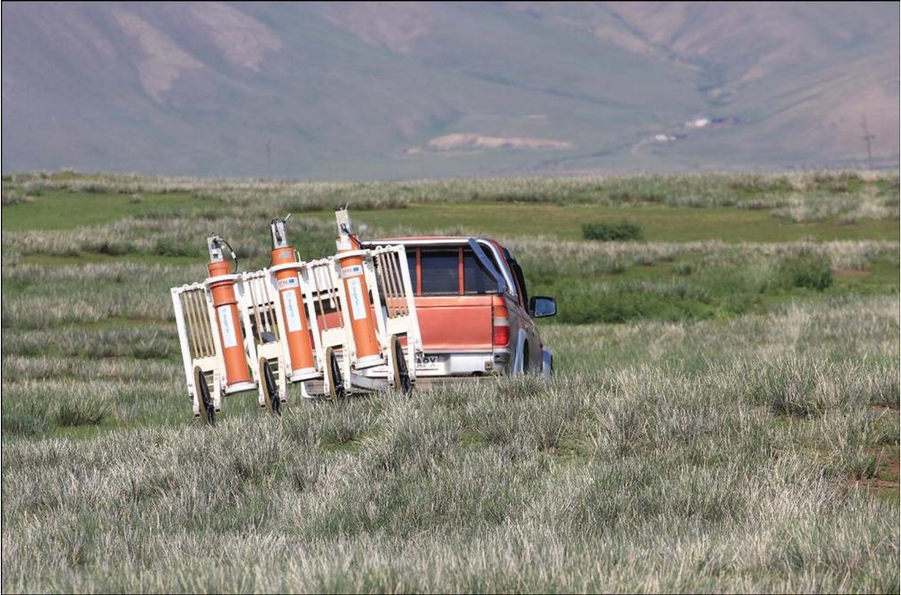
*Figure 2. The SQUID measuring system in operation at Karakorum (photograph by J. Bemmann).*
