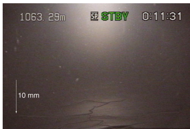
Fig. 19. Looking from below onto the base of the ice with grain boundaries visible. Picture upside-down. Slight turbidity in the water backscatters light. The contrast in this image has been enhanced digitally.
