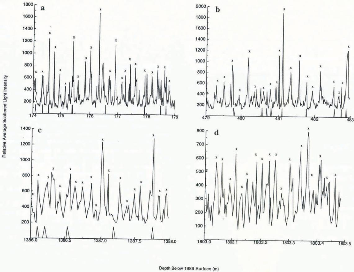
Fig. 5. Seasonal dust peaks as recorded at various depths along the GISP2 ice core. a, b and c were measured with a photomultiplier and d was measured with a photodiode. The average measuring increments in millimeters for a, b, c and d were 8, 11, 17 and 3, respectively. The × indicates the position of spring/summer dust peaks as determined by D. Meese by correlation with visual stratigraphy and ECM (Meese and others, 1994). The triangular markings on the horizontal axis show core breaks.
