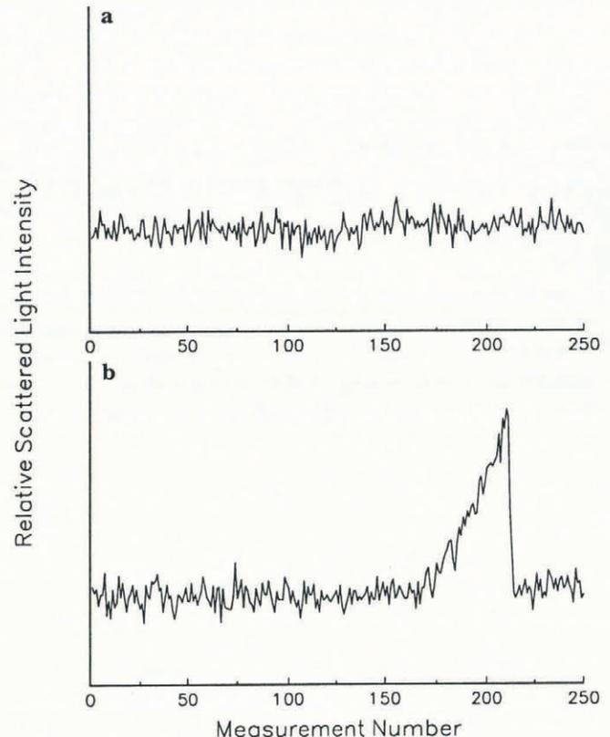
Fig. 4. a. Normal, steady, fluctuating trace as seen on the computer monitor. The trace is the result of 250,  $90^\circ$  scattered light-intensity measurements carried out in a 10 s interval. b. Unsteady trace showing the effect of a very large particle passing through an unexpanded laser-light beam.
