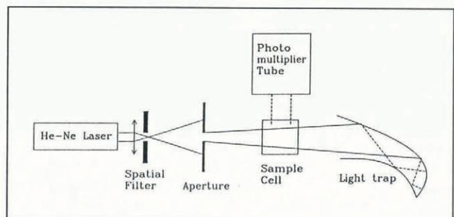
Fig. 3. Optical system for measuring 90° scattered-light intensity.
