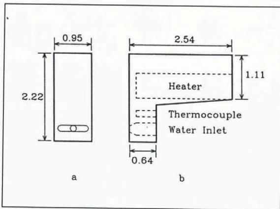
Fig. 1. Schematic diagram of ice melter: a. Front view; b. Side view, showing the cylindrical cavities for the heater and thermocouple. All dimensions are in centimeters.
