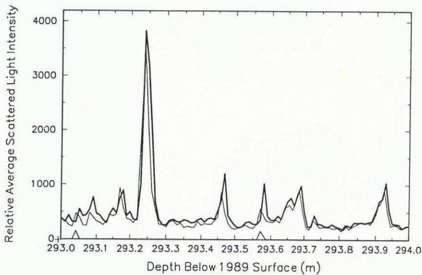
Fig. 6. Two traces recording the average 90° scattered laser-light intensity measured along parallel grooves of the same 1 m section of ice. Any difference between the two curves can be accounted for by the fact that it is impossible to melt the two grooves in exactly the same way.
