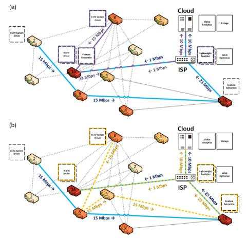
Fig. 11. Alternative placements for the second chain (links are annotated with the bandwidth allocated to chain traffic flows).
