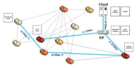
Fig. 9. Best placement for the first chain (links are annotated with the bandwidth allocated to chain traffic flows).
