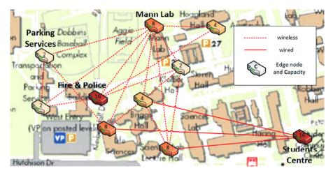
Fig. 2. Example Edge infrastructure at UC Davis (Ning et al. 2019).
