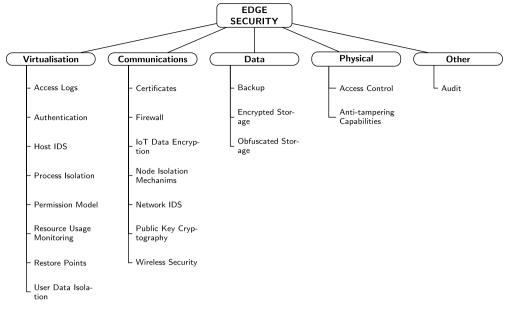
Fig. 1. Security capabilities for Edge computing.
