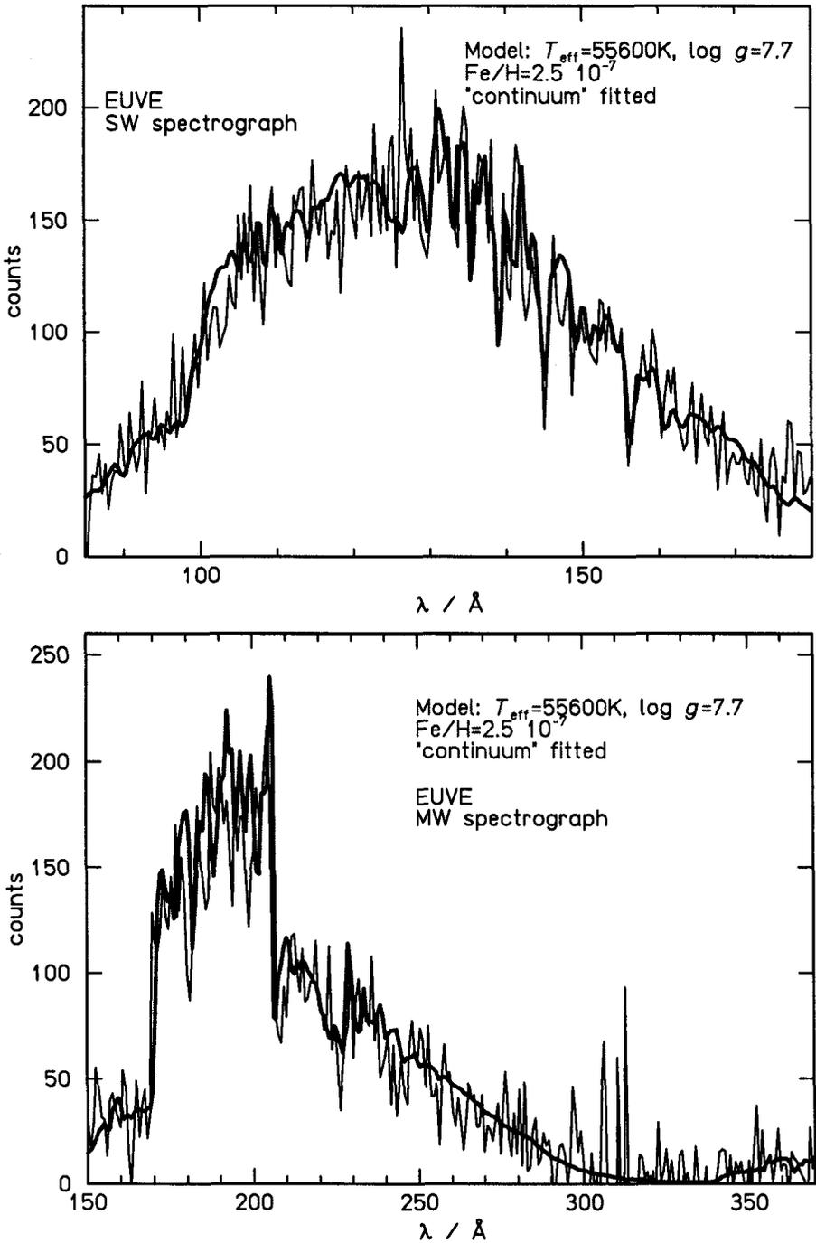
FIGURE 1. The SW (top) and MW (bottom) spectrum of PG 1234+482 is compared to a synthetic spectrum for  $T_{\text{eff}} = 55,600 \text{ K}$ ,  $\log g = 7.7$ , and  $\text{Fe}/\text{H} = 2.5 \cdot 10^{-7}$
