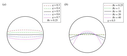
FIGURE 5. (Colour online) Fluid separation lines in branched tube flows. The cross-section is the same as that in figure 4. (a) Separation lines for flows at Re = 0.25 with different branch flow ratios; (b) separation lines for flows at different Reynolds numbers with a fixed branch flow ratio q = 0.5.
