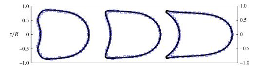
FIGURE 2. (Colour online) Steady profiles of an initially spherical capsule with a NH membrane in a uniform tube flow (a/R = 0.9, Re = 0.125, B = 0) for Ca = 0.02, 0.05, 0.1 (from left to right). Black solid lines correspond to the present model with a membrane mesh of 32 768 flat triangular elements connecting 16 386 nodes. The results are compared to the ones obtained by Hu *et al.* (2012) using a boundary element method (square symbols).
