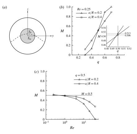
FIGURE 13. (a) Illustration for the definition of the momentum ratio. The dash line is a fluid separation line (for q = 0.5, Re = 20), which divides the cross-sectional area of the capsule (shaded circle) into two regions ( $S_b$  and  $S_m$ ) covered by fluid elements that finally enter the side branch and downstream main tube, respectively. Momentum ratios of capsules with a/R = 0.2 and 0.4 as a function of (b) q at Re = 0.25, (c) Re at q = 0.5.
