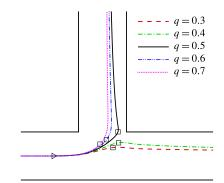
FIGURE 6. (Colour online) Effect of branch flow ratio q on the capsule trajectories (R = 0.4, Re = 0.25, Ca = 0.5). The triangle denotes the position where the bifurcation starts to affect the capsule motion. The squares label the centre of mass positions where the capsule maximum principal tension are the largest (see figure 9).
