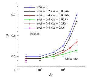
FIGURE 12. (Colour online) Phase diagram: critical branch flow ratio as a function of the tube Reynolds number for capsules with different sizes and membrane shear elasticity. For  $q > q_c$ , the capsule flows into the side branch.
