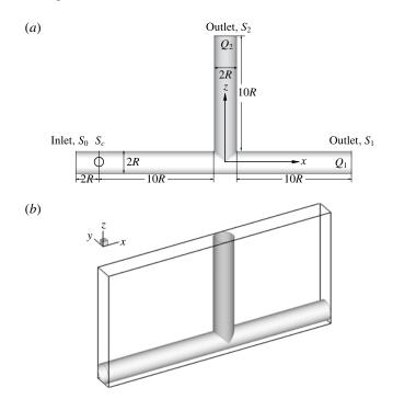
FIGURE 1. (a) Geometry of the branched tube. (b) Geometry of the computational domain.
