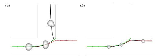
FIGURE 11. (Colour online) Effect of capsule size on its trajectory for Re = 20, q = 0.56, Ca = 0.1: (a) a/R = 0.4, (b) a/R = 0.2. The streamline legend is the same as in figure 10.
