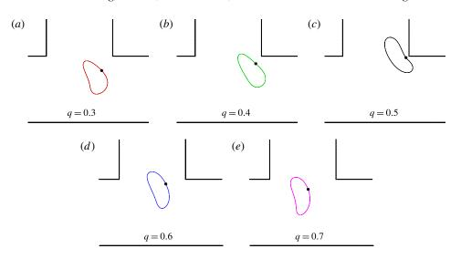
FIGURE 9. (Colour online) Capsule profiles in the *xz*-plane when the maximum principal tension reaches its peak (a/R = 0.4, Re = 0.25, Ca = 0.5). The black dots show where the principal tension is maximum.
