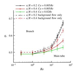
FIGURE 14. (Colour online) Phase diagram: critical branch flow ratio as a function of the tube Reynolds number for capsules with a/R = 0.2 and 0.4, Ca/Re = 0.005. Solid lines: full fluid-structure simulations with a capsule (see figure 12); dash lines:  $q_{cm}$  from the background flow only.
