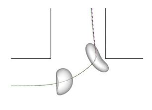
FIGURE 3. (Colour online) Trajectories of a capsule (a/R = 0.4) flowing in the branched tube at Re = 0.25, Ca = 0.5, q = 0.5. Different grid resolutions are used:  $\Delta x = 0.05R$  (dashdot line),  $\Delta x = 0.04R$  (solid line),  $\Delta x = 0.031R$  (dash line).
