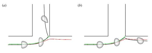
FIGURE 15. (Colour online) Effect of membrane shear elasticity on the capsule trajectory for Re = 20, q = 0.53, a/R = 0.4: (a) Ca = 0.4, (b) Ca = 0.1. The streamline legend is the same as in figure 10.
