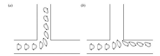
FIGURE 7. Effect of flow split ratio on the path selection of a capsule (a/R = 0.4, Re = 0.25, Ca = 0.5). The profiles are plotted in the *xz*-plane. The black dots are attached to two material points of the capsule membrane. The profiles are shown at Vt/R = 4.16, 4.8, 5.44, 6.08, 6.72, 8, 9.28, 10.56, 11.84. (a) q = 0.6, (b) q = 0.4.
