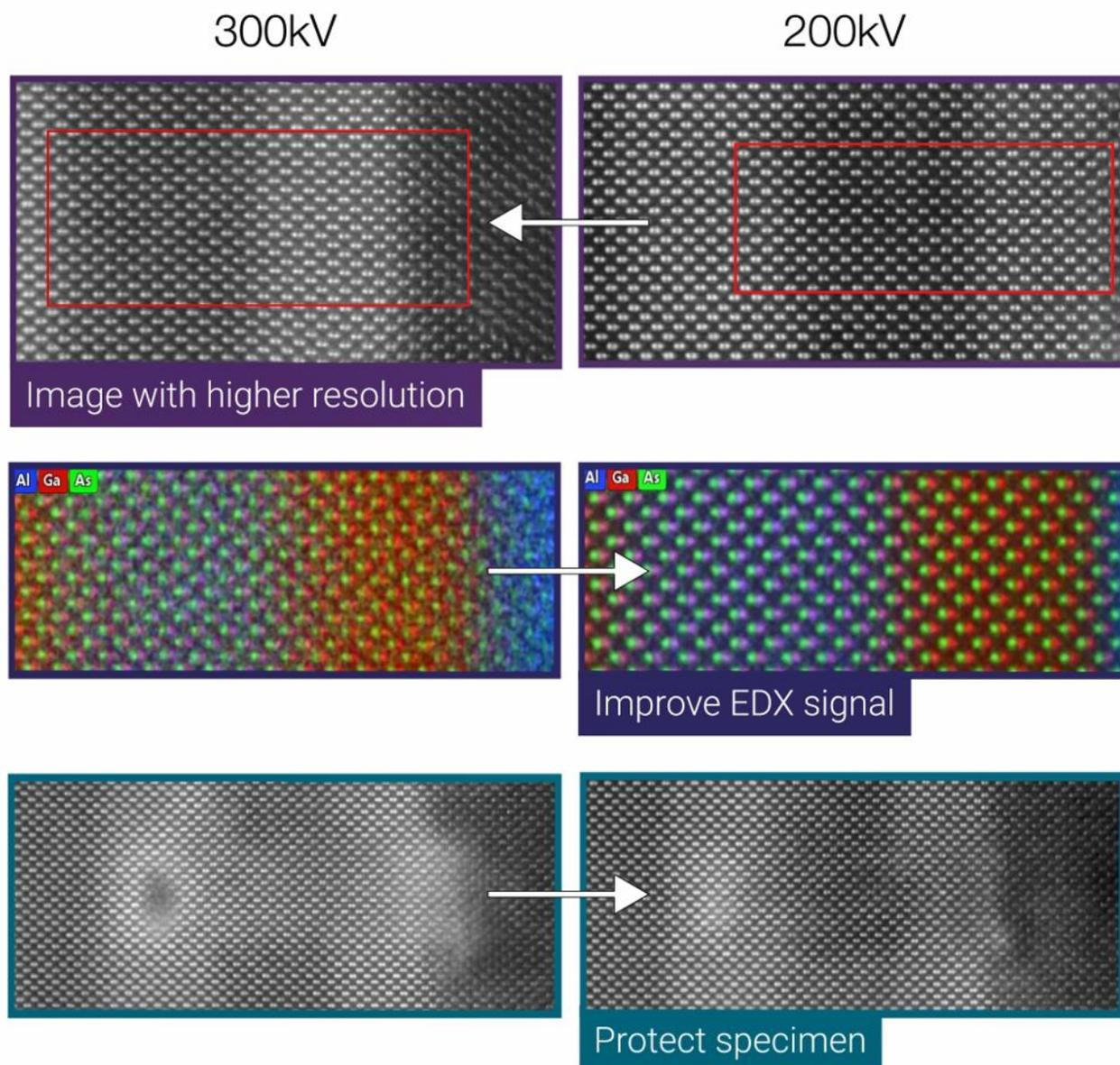
**Figure 1.** Al-Ga-As multilayer sample courtesy of J. Zweck, University of Regensburg; data collected by Cigdem Ozsoy-Keskinbora. The combined 300kV and 200kV imaging and EDX mapping experiment was performed in less than 1 hour.
