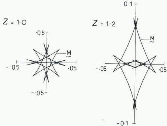
Fig.5. The metacentric locus  $M$  for a rectangle computed for a relative density  $\lambda = 0.828$  and aspect ratio  $Z = 1.0$  and  $1.2$ . The thickness is taken as unit length; note the small size of  $M$ .
