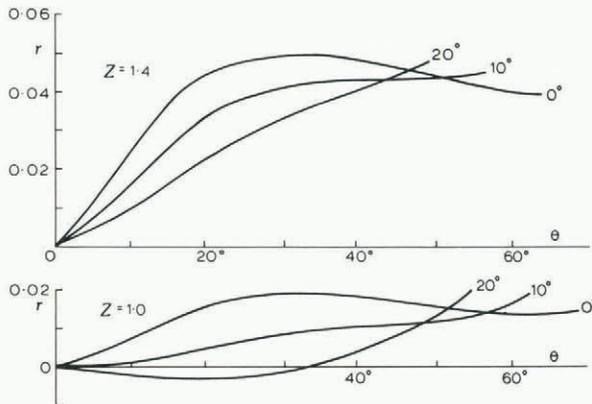
Fig.8. The righting arm  $r$  (see Fig. 1) as a function of attitude  $\theta$  for trapezia of different aspect ratio  $Z$  and side inclination  $\phi$  (shown in degrees against each curve). The normal density distribution of Weeks and Mellor (1978) was used.  $r$  is measured in units of the thickness of the trapezium.
