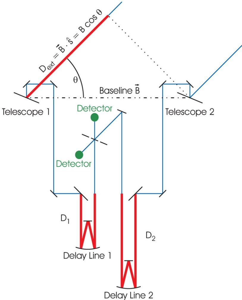
**Figure 1.** Schematic drawing of the light path through a two-element interferometer. The external delay  $D = \vec{B} \cdot \hat{s}$  is compensated by the two delay lines. The pathlengths  $D_1$ ,  $D_2$  through the delay lines are monitored with laser interferometers. The zero-order interference maximum occurs when the delay line positions are such that the internal delay  $D_{\text{int}} = D_2 - D_1$  is equal to  $D$ .
