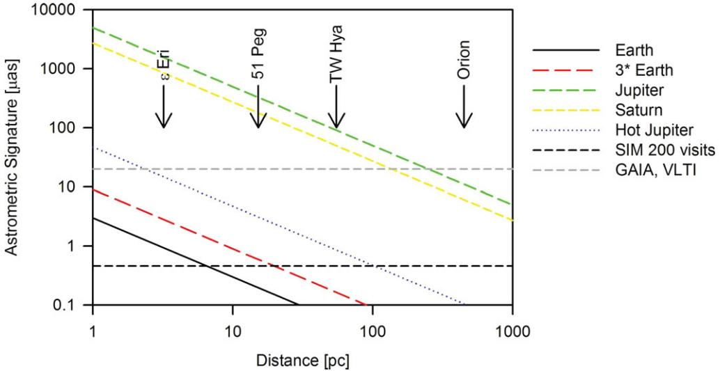
**Figure 2.** Astrometric signature (semi-amplitude) for five sample planets orbiting a Solar-mass star, as a function of distance. Anticipated detection limits for ground-based (VLTI PRIMA) and space-based (Space Interferometry Mission) instruments are also shown. Adopted from Quirrenbach (2003).
