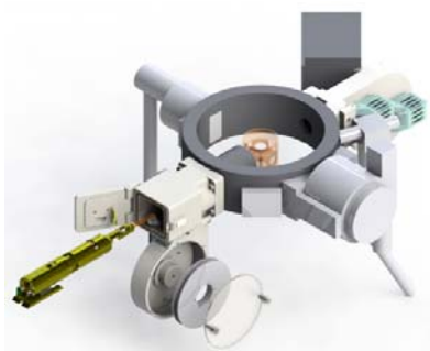
Figure 1. Section view of GridStage™ reel-to-reel sample handling system and high speed rastering cartridge installed on JEOL 1200EX microscope column. The exploded view shows a reel. Tape advances from the feed reel (left) to the take-up reel (right).
