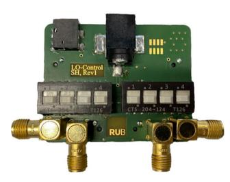
**Fig. 7.** Photograph of the control board. It generates the necessary supply voltages from 5 V and 12 V, respectively. To change the divider value double-throw dip switches are located on the PCB. SMA connectors are utilized to supply the reference frequency and probe the frequency divider's output.
