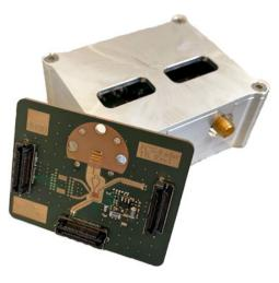
Fig. 1. Photograph of built LO module with the RF frontend highlighted.
