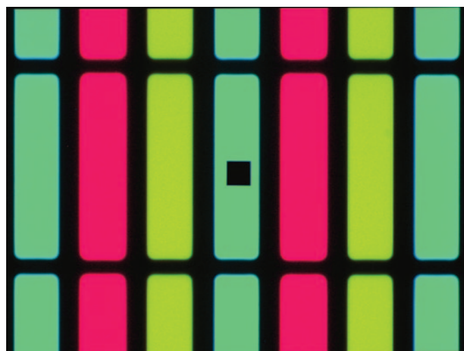
Figure 2: When imaging a sample with a microspectrophotometer, the black square in the center of the image is the entrance aperture for the spectrophotometer. The user simply moves the sample stage so the black square is superimposed over the area to be measured as with this organic light emitting diode (OLED) display.
