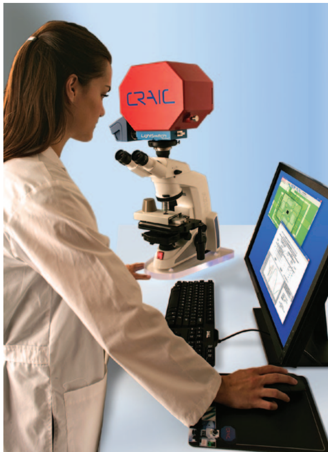
Figure 1: A microspectrophotometer integrated with a microscope can analyze the UV-visible-NIR region.
