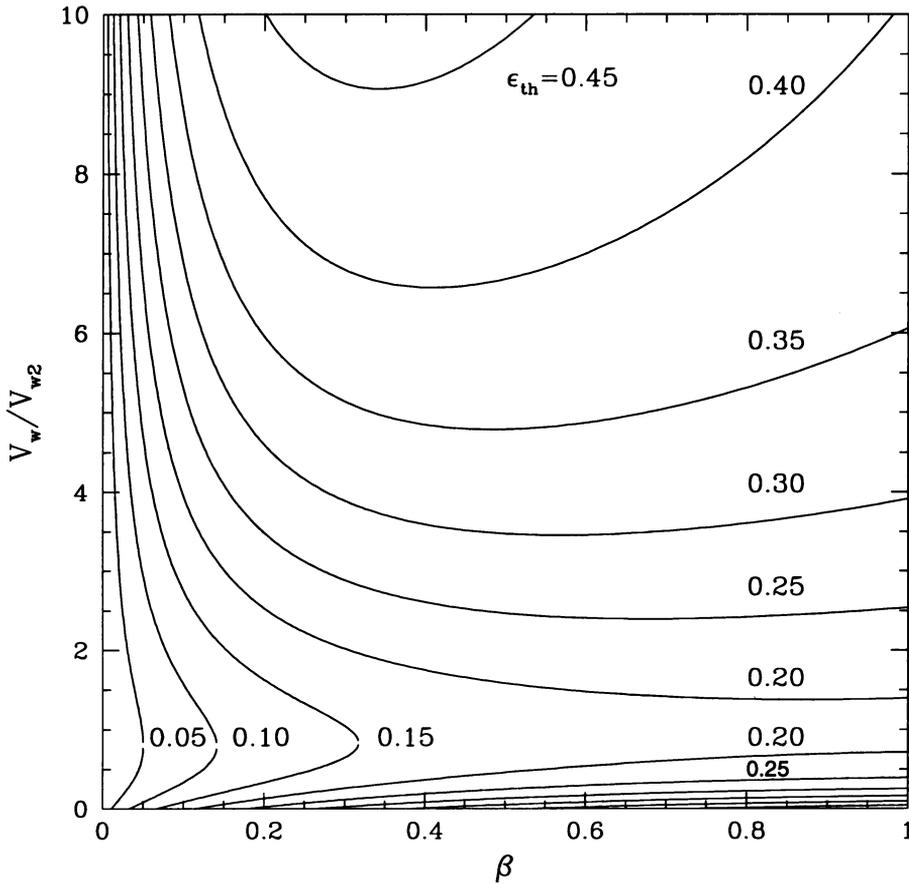
*Figure 4.* Efficiency of thermalization of pre-shock wind kinetic energy. Contours of equal thermalization efficiency  $\epsilon_{th}$  are shown in terms of the ratio of wind momentum loss rates,  $\beta$ , and the ratio of wind speeds.
