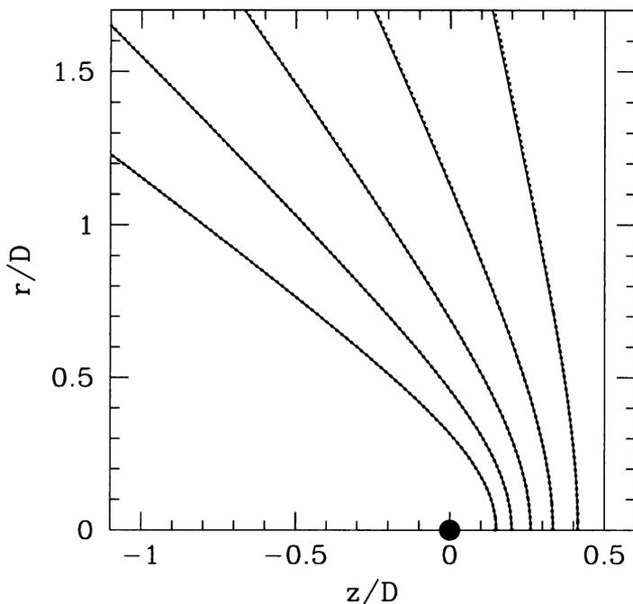
*Figure 3.* Solutions to the two-wind collision problem. The two wind sources are separated by a distance  $D$ , so that the weaker source is at the origin, while the stronger source is off the right edge of the graph at  $z/D = 1$ . Moving from right to left, the solutions correspond to  $\beta = 1, 0.5, 0.25, 0.125, 0.0625, 0.03125$ .
