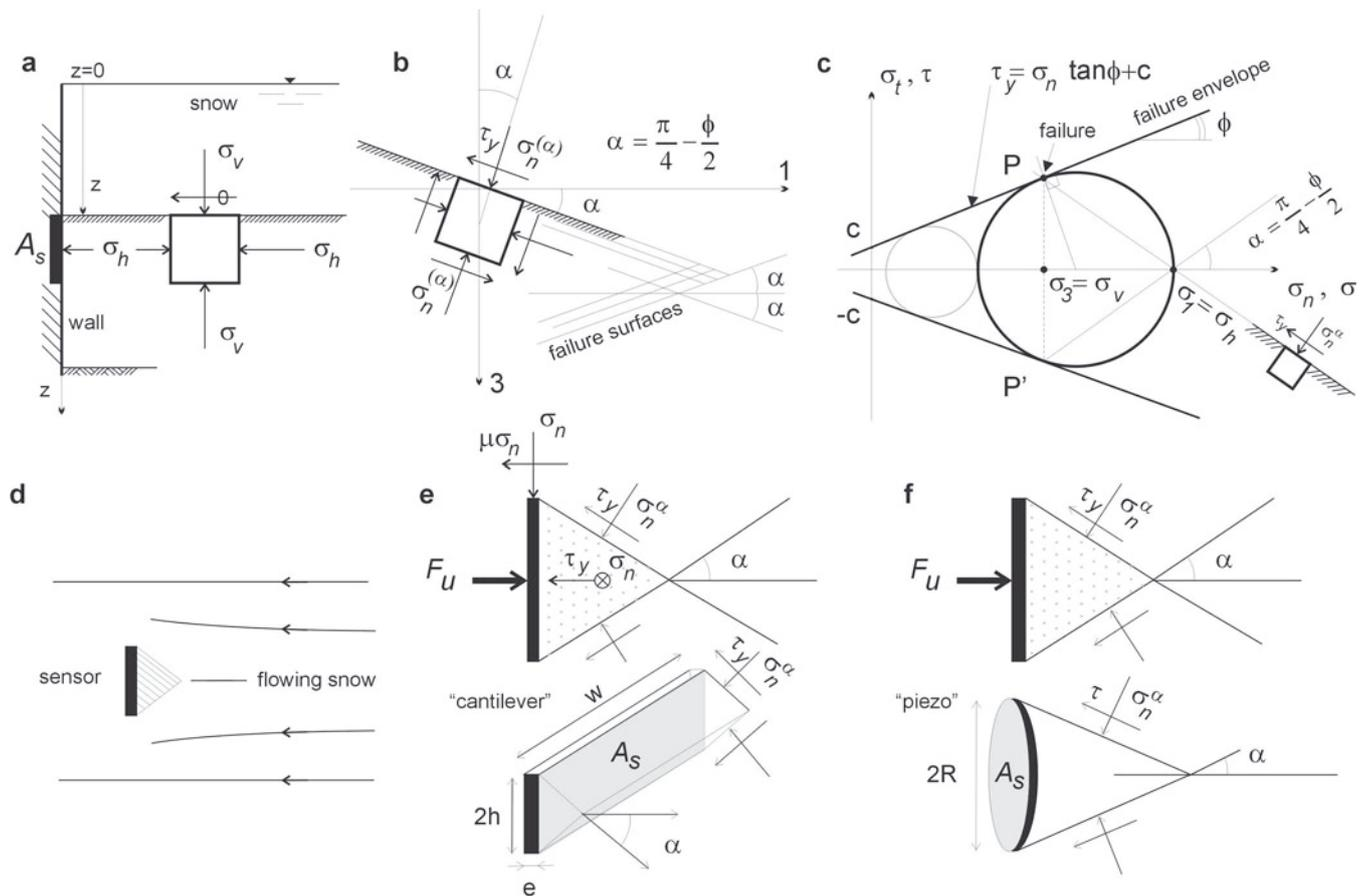
**Fig. 14.** Local shear failure approach. (a) Passive lateral earth pressure on a vertical wall immersed in snow (reference case). (b) Failure surface orientation  $\alpha$ . (c) Passive pressure at failure (upper equilibrium; large circle) given by the Mohr–Coulomb criterion. (d) Snow deposited on the sensor surface: (e) cantilever sensor, (f) piezoelectric sensor.
