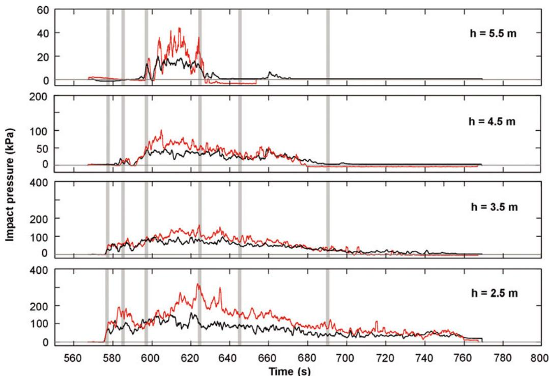
**Fig. 9.** Avalanche 8448. Time-averaged impact pressures along the pylon height using  $T=1$  s for the time averaging. The red curves are the cantilever sensor pressures, and black curves are the piezoelectric sensor pressures. Vertical gray bars show characteristic times for which vertical profiles of pressure are plotted in Figure 10.
