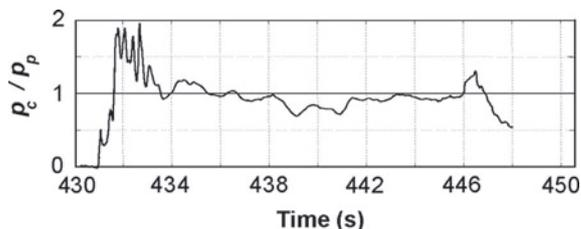
**Fig. 5.** Observed ratio of impact pressures (cantilever over piezo),  $p_c/p_p$ , vs time for avalanche 2009-003 at 1.5 m for the whole avalanche duration. There are two distinct regimes with a ratio of  $\sim 1.5$ –2.0 in the head and 1.0 in the body and tail of the avalanche.
