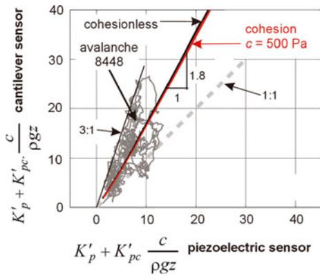
**Fig. 16.** Normalized horizontal pressure for cantilever vs piezo measurements (gray scattering points) using  $z=3$  m (as estimated from pressure profiles in Fig. 10) and  $\rho=400$  kg m<sup>-3</sup>. Model results are given by the continuous black line with a slope of  $\sim 1.8$  for  $\mu=0.4$ .
