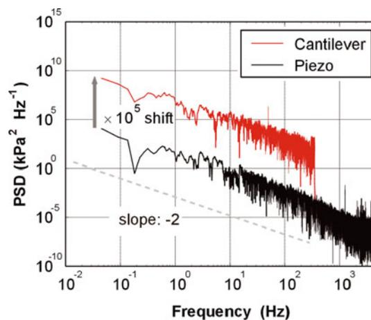
**Fig. 7.** Avalanche 2009-003. PSD of impact pressure at 1.5 m computed over the entire avalanche duration. The cantilever power spectrum is shifted up by five decades ( $\times 10^5$ ) for better legibility. Its frequency cut-off above  $\sim 430\text{ Hz}$  is due to necessary regularization in the deconvolution. The frequency dependence is shown by the gray line with a slope of  $-2$ .
