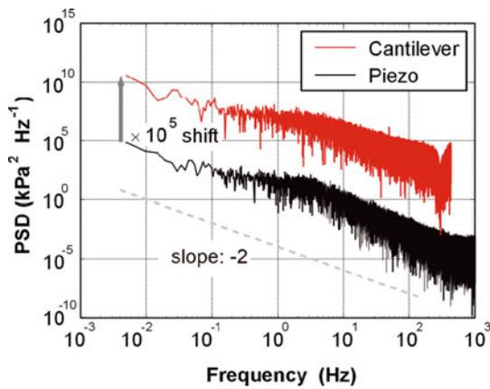
**Fig. 13.** Avalanche 8448. Power spectra density (PSD) of impact pressure at 2.5 m computed over the entire avalanche duration. The cantilever powder spectrum is shifted vertically by  $10^5$  for better legibility. The frequency dependence is shown by the gray line with a slope of  $-2$ .
