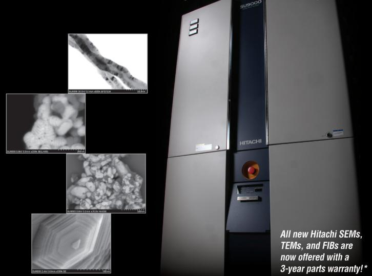
Hitachi's latest FE-SEM system, Model SU9000, is designed for ultra-high-resolution imaging, even for beam-sensitive specimens and advanced semiconductor devices that require stable observation at maginifications up to 3,000,000 times.
