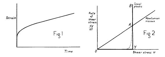
when the transient flow has died away. Transient flow is considerable only after a relatively rapid change of the stress; we can disregard it in dealing with the simplest features of glacier flow.
