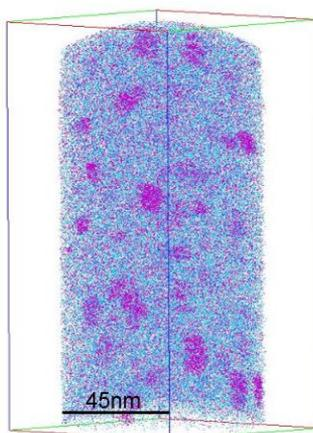
**Figure 1.** Mg-based dielectric nano-particles (pink) surrounded by silica matrix (blue).
