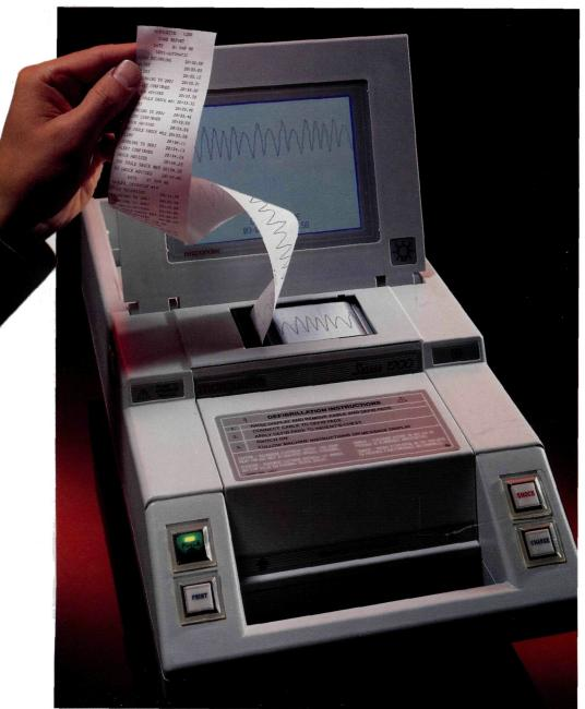
Marquette's 1200 Responder™ semi-automatic defibrillator begins to analyze the patient's heart signals from the instant the power is switched on. It continuously interprets the heart's rhythms, using a sophisticated and field-tested computer analysis program and quickly guides the operator to provide life-saving defibrillation when appropriate.
