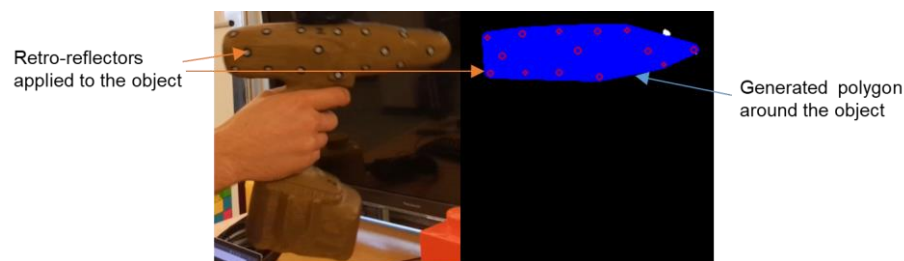
Figure 3. Reflectors and ICP on drill prototype
