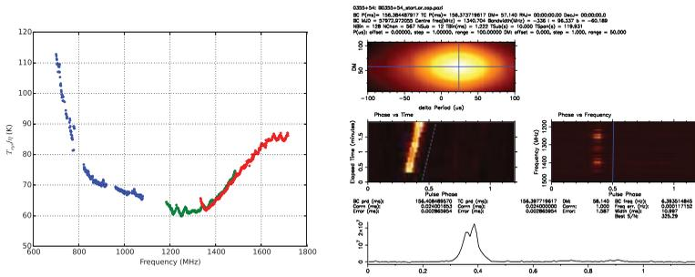
**Figure 1.** Early results of a PAF system at Effelsberg 100 m telescope. The left sub-figure represents the system temperature over efficiency of PAF’s central beam. From left to right are the results for 1200 MHz, 1450 MHz and 1800 MHz bands separately. The right sub-figure shows the observation of PSR J0358+5413 (B0355+54) with the same beam.
