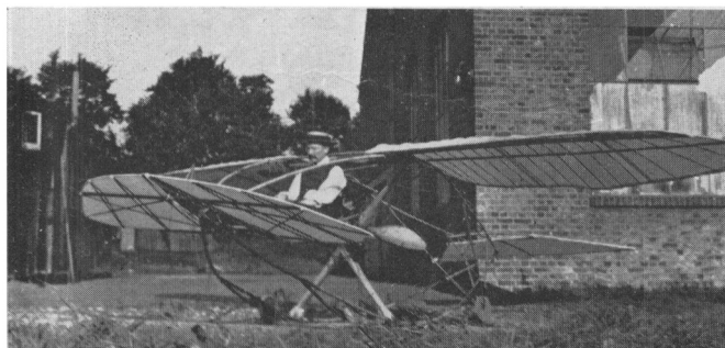
Major Baden-Powell's monoplane The Midge . Structure: American elm, streamlined where exposed. Four main members of bamboos, jointed with short steel connections. Double skids, solid wooden wheels on steel forks with spiral springs. Planes: Elevator 30 sq. ft. on universal joint. Main plane 90 sq. ft. bamboo frame. 25 ft. span, 3 ft. 10 in. chord. Surface pegamoid cloth. Tail plane 20 sq. ft. on bamboo frame. Engine 12 h.p. Buchet. Wooden propeller 5 ft. 6 in. diam. Total weight, including pilot, 350 lb. Price complete, including engine and all fittings, £120. Date 1910.
