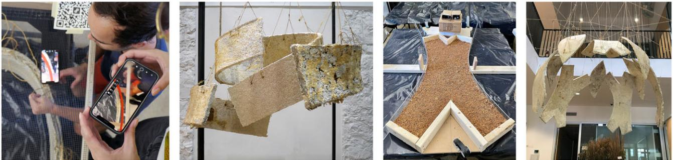
**Figure 2.** Processes and prototypes that preceded the design, cultivation and installation of Phoenix. On the left, bending living sheets guided by augmented reality for the Myco-Chandelier. On the right, cultivating non-rectangular sheets with flexible formwork for the hanging Myco-Pod. Photos by Jonathan Dessi-Olive.
