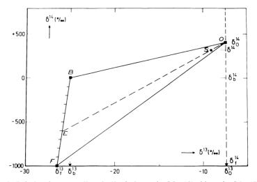
Fig 2. Relation between  $\delta^{13}$  and  $\delta^{14}$  of clean air  $CO_2$  (O), biogenic  $CO_2$  (B) and fossil fuel  $CO_2$  (F). S refers to an arbitrary atmopsheric  $CO_2$  sample. The fraction of contaminating  $CO_2$  (f+b) is presented by OS/OE, while f/b=BE/FE. The isotopic compositions of B and F are arbitrarily chosen.
