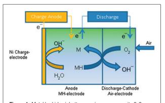
Figure 4. Metal hydride air battery can increase capacity 2–3 times relative to NiMH batteries. To avoid degradation issues of an air cathode during charging, a third Ni electrode has been added.
