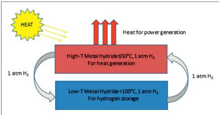
**Figure 5.** Metal hydride thermal energy storage. Heat irradiates the high-temperature (HT) bed, which releases 1 atm H<sub>2</sub> to the low-temperature bed for storage until heat is needed. When the sun (heat source) is absent, H<sub>2</sub> diffuses back to the HT bed, a chemical bond is formed between the metal and hydrogen, and heat is released for power generation.
