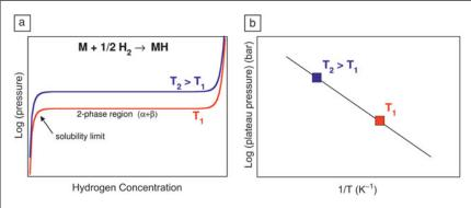
**Figure 2.** Metal hydride basics. (a) The pressure-composition isotherm for two temperatures  $T_2 > T_1$ . (b) The slope of the van't Hoff plot yields the enthalpy  $\Delta H$  for the reaction.
