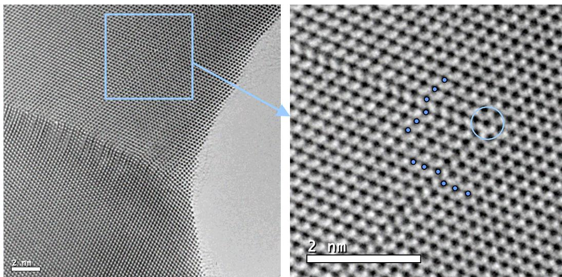
Fig. 1. Cs-corrected HR-TEM image of gold in  $\langle 110 \rangle$  direction at 300kV. In the upper crystal two twins touch each other under an angle of  $60^\circ$ . The area of interest is magnified in the right image. The blue dots indicate the atomic positions across the twins. The point, in which the twins are touching each other, can be clearly resolved, exemplifying the benefits of an image Cs-corrector.
