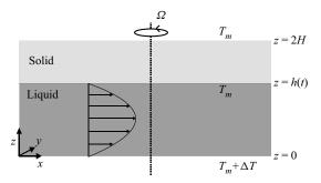
Figure 1. A vertical cross-section of the geometry considered. The size of the domain is  $L \times L \times 2H$ , with aspect ratio A = L/2H. The bottom surface is maintained at a higher temperature than the interface. No-slip and no-penetration conditions for the fluid velocity are imposed at the bottom boundary and the evolving interface, and periodic boundary conditions are imposed in the horizontal.
