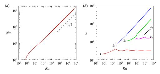
FIGURE 9. (a) The upper bound of Nu versus the Rayleigh number Ra with  $Nu \leq 0.055Ra^{1/2}$  in the asymptotic regime. (b) The bifurcation diagram of critical wavenumber  $k_m$  versus the Rayleigh number.
