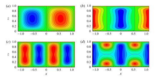
FIGURE 3. At Ra = 4468.8, the first mode (a)  $\psi_1$  and (b)  $\theta_1$  and the new second mode (c)  $\psi_2$  and (d)  $\theta_2$ .
