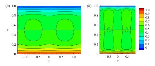
FIGURE 4. (a) The optimal background field  $\tau$  plotted at Ra = 2000 and (b) the non-optimal 1-mode solution at Ra = 20000.
