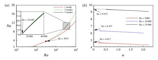
FIGURE 5. (a) The Nusselt number Nu versus the Rayleigh number Ra at fixed aspect ratio  $L = 2\sqrt{2}$ . (b) Nu versus  $\alpha = 2\pi/L$ .
