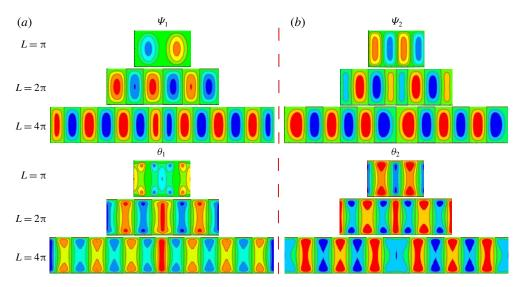
FIGURE 6. (a) The first mode  $(\psi_1, \theta_1)$ ; (b) the second mode  $(\psi_2, \theta_2)$  at  $Ra = 10^4$  (only two critical modes are present for this Ra).
