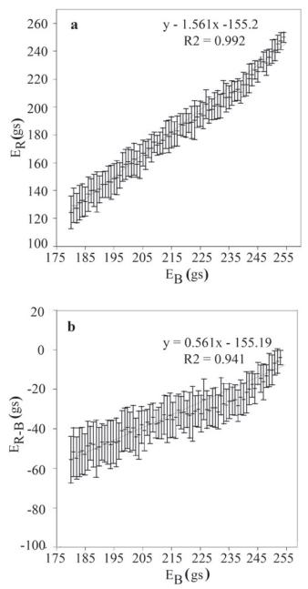
**Fig. 4.** (a) Sony CCD red channel excitation ( $E_R$ ) as a function of blue channel excitation ( $E_B$ ) for gs values  $100 < E_R < 255$  and  $180 < E_B < 255$ . (b) The difference in red and blue channel response as a function of blue channel excitation.
