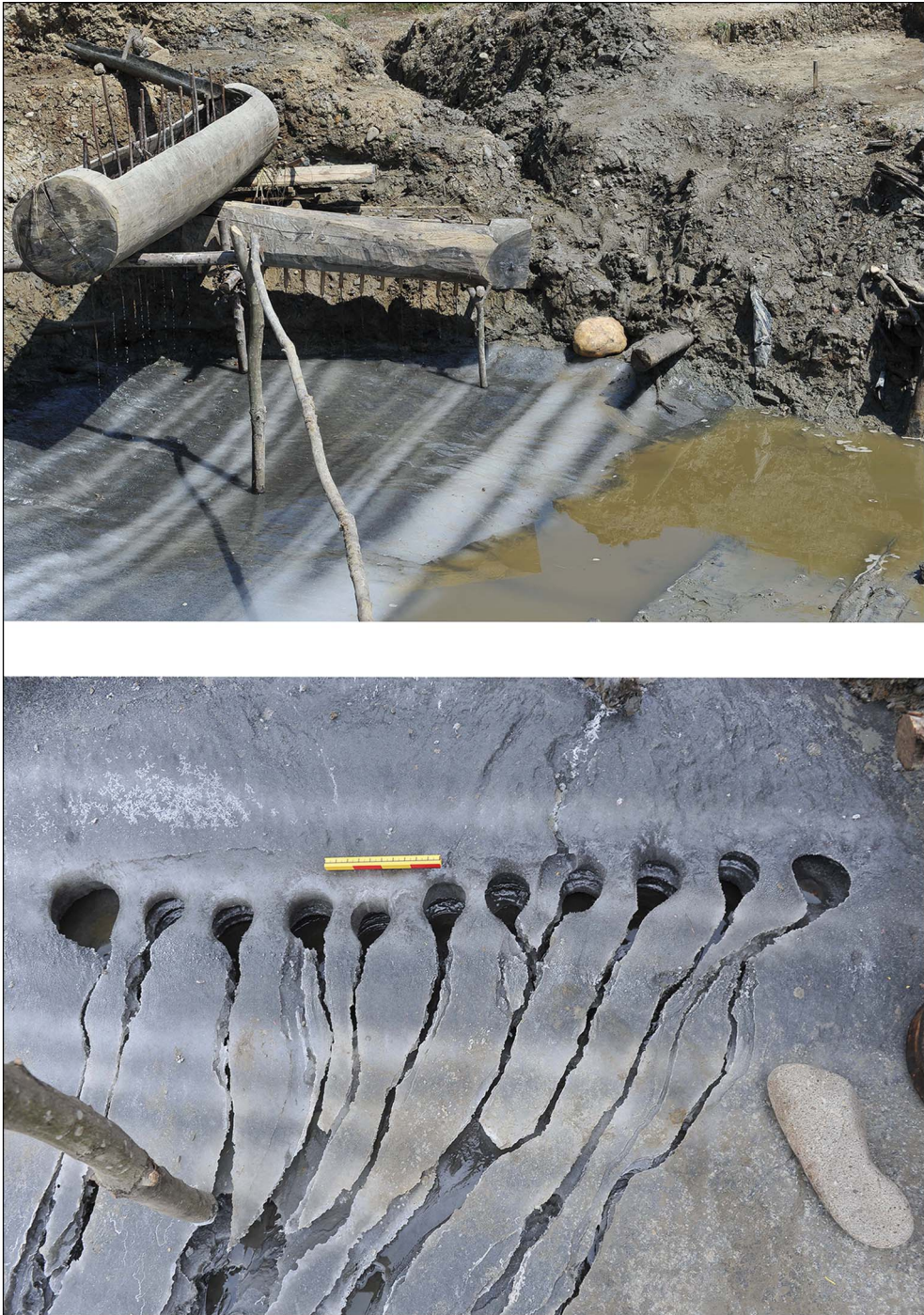
Figure 8. Top) experimental troughs set up over the rock salt; bottom) depressions formed in the rock salt after water was allowed to drip onto it (figure courtesy of the National Museum of the Eastern Carpathians).
