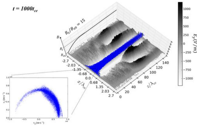
**Figure 3.** Composite overview of 3D VSim PIC simulation results in an  $x$ - $z$  plane ( $y = 0$ ) showing magnetic compression of an electron beam and subsequent cyclotron-maser emission in the X-mode at  $t = 1000t_{ce}$ . The electron PIC particle trajectory is also overlaid (blue scatter plot) along with the corresponding velocity distribution over the simulation volume at  $t = 1000t_{ce}$ .
