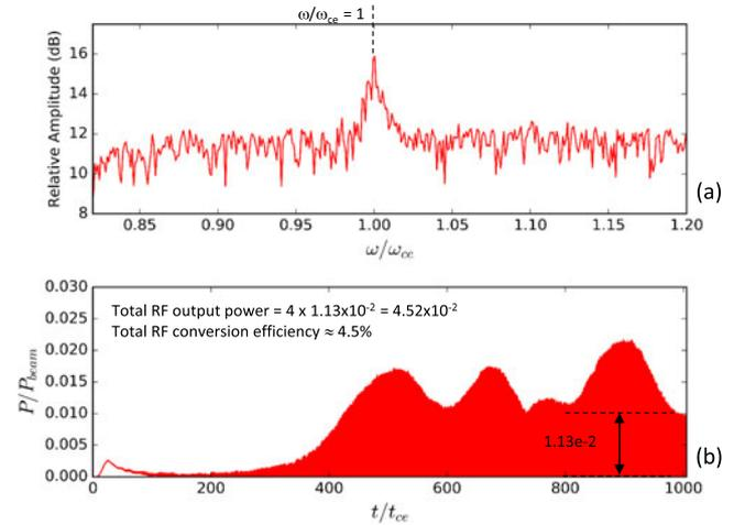
**Figure 4.** 3D VSim PIC simulation results showing (a) the spectrum of EM emission at  $z = 86\lambda_{ce}$  and (b) the transverse Poynting flux in a  $y$ - $z$  plane displaced from the electron beam.
