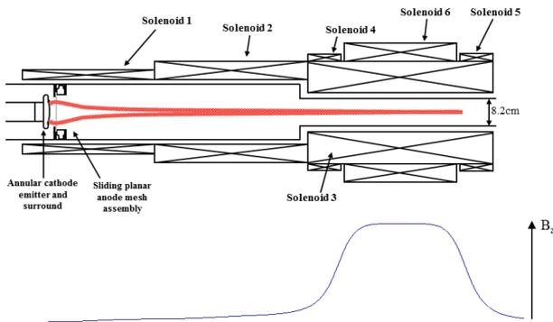
**Figure 5.** Diagrammatic overview of the experimental setup showing the magnetic coil configuration, electron gun and the convergent axial magnetic field profile with peak-plateau region for cyclotron resonant energy transfer.
