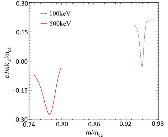
**Figure 2.** Imaginary part of the refractive index as a function of frequency for a mean beam energy of 100 keV and a thermal spread of 1 keV, and a mean beam energy of 500 keV and a thermal spread of 5 keV. The magnetic field ratio is taken to be 20.
