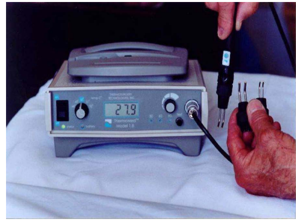
Fig. 1. ThermoMed™ 1.8. It is shown heating up on its way to 50 °C. The three different sized applicators are shown, the thinner one for thin skin, such as on the face, the largest when deeper penetration is needed on the extremities. From David JR, personal photos.
