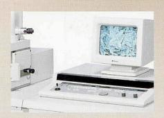
All have windows mouse-based computer controls or traditional automated controls, or both, to provide access to all SEM func-
