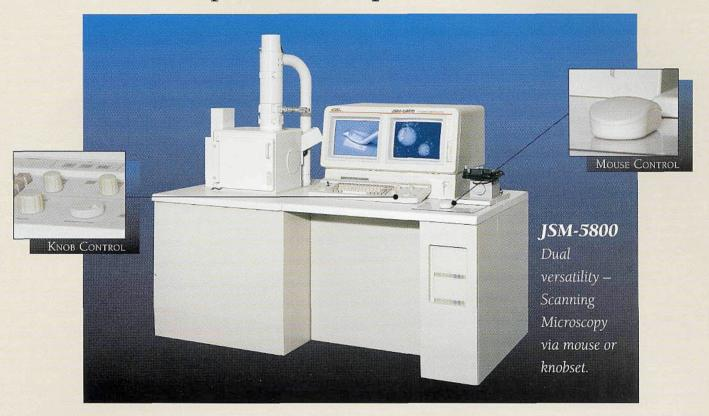
■ Large Specimen Stage ■ High/low vacuum capability ■ Super Conical Objective Lens for high resolution
