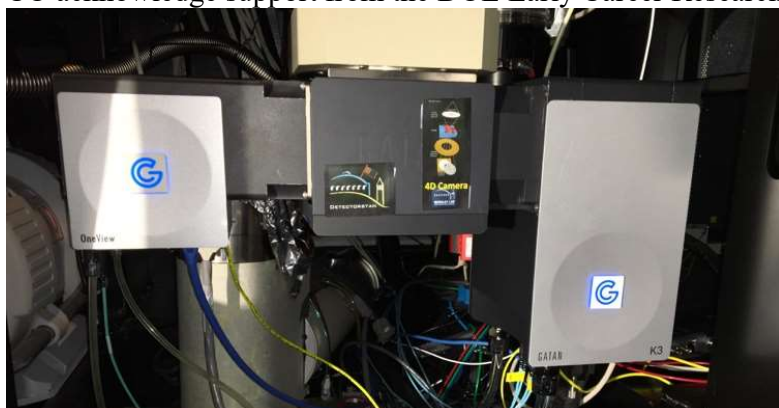
Figure 1. Optical photograph of installed detector system
