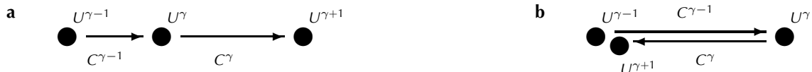
Fig. 1. Illustration of (a) undershooting and (b) overshooting for a sequence of iterates, U^{\gamma-1} , U^\gamma and U^{\gamma+1} , and corresponding correction vectors, C^{\gamma-1} and C^\gamma .
