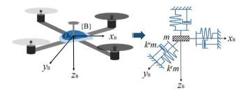
Fig. 11. Hovering UAV acts as a spring-mass-damper system.
