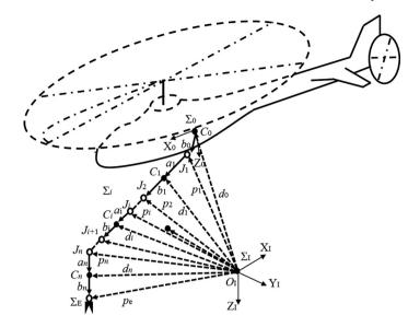
Fig. 9. Frames of AM system based on the centralized approach.
