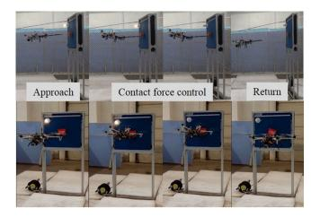
Fig. 17. The process of pressing an emergency switch.
