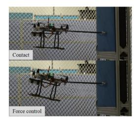
Fig. 14. The contact force control experiment with a quadrotor AM.
