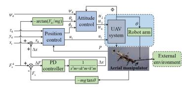
Fig. 13. Contact force control block diagram of AM.
