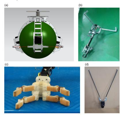
Fig. 4. Gripper examples. (a) Ball gripper, (b) Three-finger gripper, (c) Yale hand, (d) Simple gripper. Other grippers: Yale University,<sup>8</sup> University of Pennsylvania,<sup>10</sup> Utah State University,<sup>73</sup> ETH Zurich,<sup>74</sup> Johns Hopkins University,<sup>75</sup> University of Utah.<sup>77</sup>
