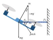
Fig. 12. An aerial manipulator contacts with a wall.
