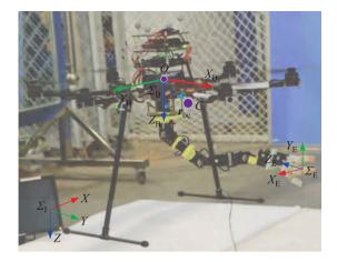
Fig. 7. Frames of AM system based on the separated approach.
