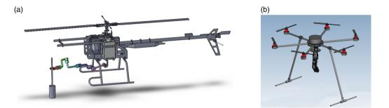
Fig. 2. Aerial manipulation examples. (a) Unmanned helicopter aerial manipulator (Yale University,<sup>8</sup> DLR,<sup>9</sup>) (b) Multirotor aerial manipulator (University of Pennsylvania,<sup>10</sup> Drexel University,<sup>11</sup>).
