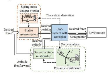
Fig. 10. Overview of the closed-loop UAV-based approach.
