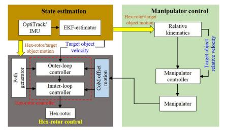
Fig. 8. Control structure of AM system based on decentralized approach.
