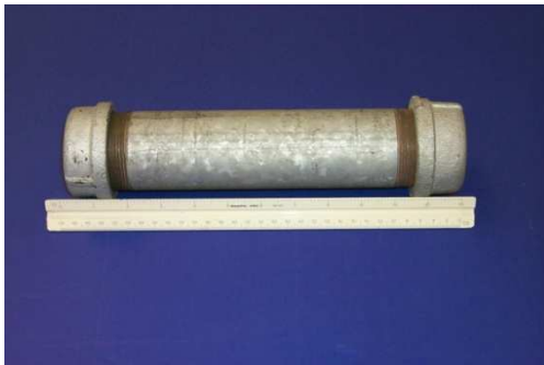
1. Example of pipe bomb used for study
