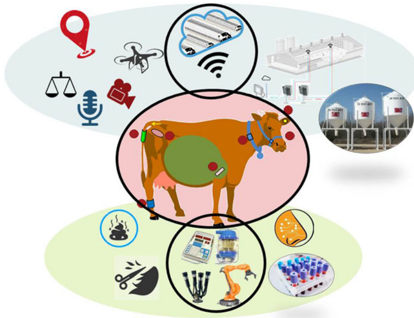
Figure 1 (colour online) Overview of sensor technologies associated with dairy animals (example is dairy cow but others could apply equally well). The red zone and individual red dots show 'At Cow' sensors, chiefly accelerometer based but also in some cases including temperature, heart rate and pH analysis. The blue zone shows 'Near Cow' sensors such as video and sound analysis, climate analysis, feed analysis, GPS and interaction with the cloud (the latter two classified as 'near' on the basis of enabling real-time analysis). The green zone shows 'From Cow' sensors that monitor products coming from the cow (milk, hair, saliva, sweat, nasal secretion, breath, faeces, etc.). The black circles represent the main technologies that are commercially available and in widespread use. A cow is shown as example; many of the technologies are also applicable to other dairy ruminants. The figure is not exhaustive.
