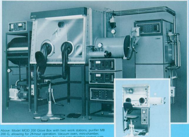
Above: Model MOD 200 Glove Box with two work stations, purifier MB 200 G, allowing for 24-hour operation. Vacuum oven, mini-chamber, moisture analyzer, oxygen analyzer, box and ante-chamber control with solid state safety device. Right: Model MB 120 or 150 single station Glove Box with integrated gas purification system.
