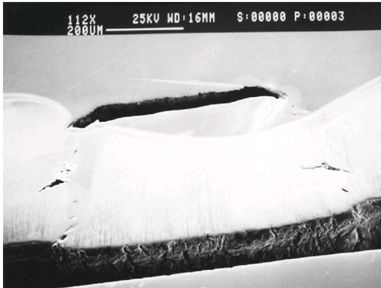
Figure 1. SEM photomicrograph of a cross-section through the pipe wall showing a typical blister crack where the material is lifted by the pressure of hydrogen.
